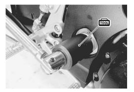
• Hold the swingarm pivot shaft (5) and remove the swingarm pivot nut (6).
