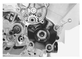
Install the starter idle gear No. 1 shaft 6, thrust washer 7, bearing 8, starter idle gear No. 1 9, washer 10, and spring washer 11.
