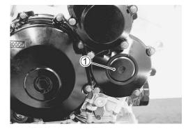
• Turn the crankshaft to bring the line (A) on the starter clutch to the index mark (B) of the valve timing inspection hole and also to bring the cams to the position as shown.
