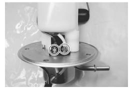
• Remove the lead wire 1, screws and fuel level gauge 2.
