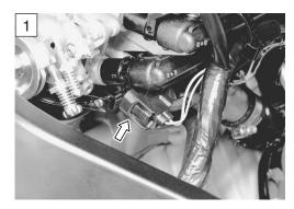
4) Disconnect the injector coupler and measure the resistance between terminals.
