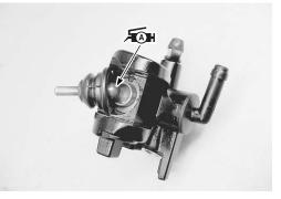
• Apply SUZUKI SUPER GREASE "A" to the push rod.
