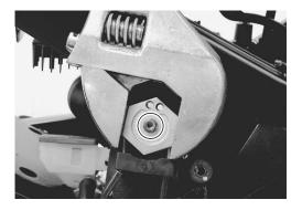
After connecting the No. 2 cable <sup>①</sup>, loosen the lock-nut <sup>①</sup> and turn the adjuster <sup>①</sup> in or out until 16 – 17 mm (0.63 – 0.67 in) of the thread length <sup>●</sup> on the cable adjuster cam be provided and tighten the lock-nut <sup>①</sup>.
