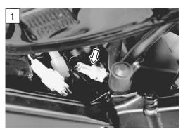
4) Disconnect the CKP sensor coupler and measure the resistance.
