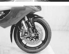
• Tighten two axle pinch bolts on the left front fork leg to the specified torque.
