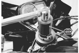
• Remove the dust seal cover ①, dust seal ②, steering stem upper bearing inner race ③ and bearing ④.
