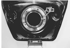
• When installing the fuel pump assembly, first tighten all the fuel pump mounting bolts lightly and then to the specified torque, in the ascending order of numbers.
