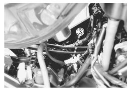
• Place the measuring cylinder and insert the fuel hose end into the measuring cylinder.
